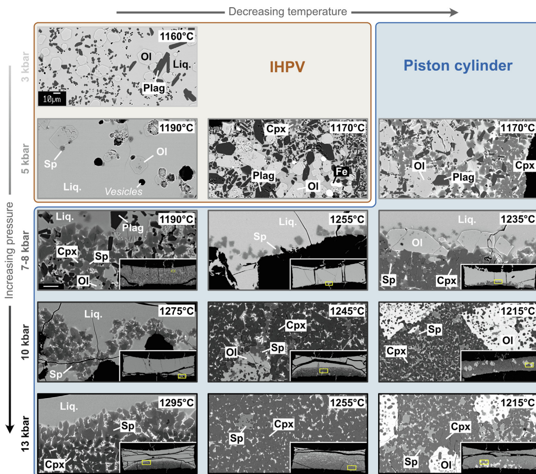
Fig. 5. Representative BSE images of selected high-pressure experiments. Temperature decreases towards the right and pressure increases towards the bottom. The 10- \mu m scale bar in the top left panel applies to all images except B1421 (middle row, left column), which is 2x magnified (see 10- \mu m scale bar in that panel).
